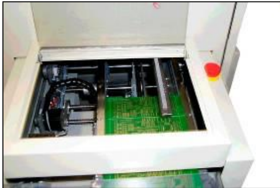
1. PCB takeover onto the inlet conveyor
