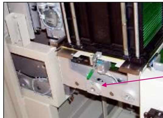
3. PCB will be passed underneath the magazine table.
