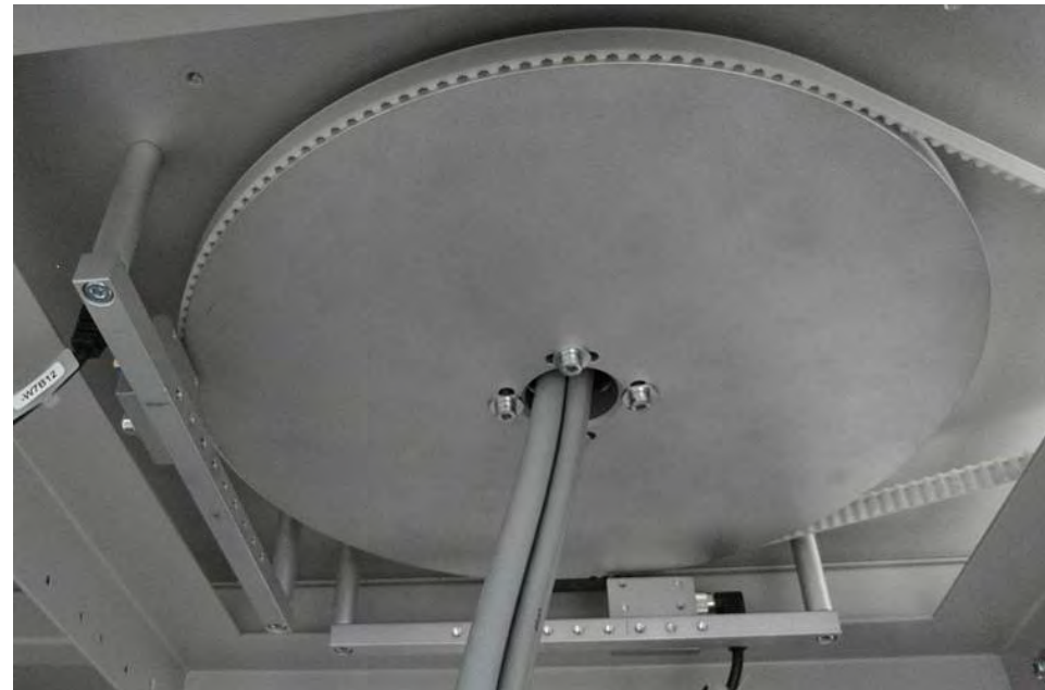
Drive pulley of the turn table with cable bushing
