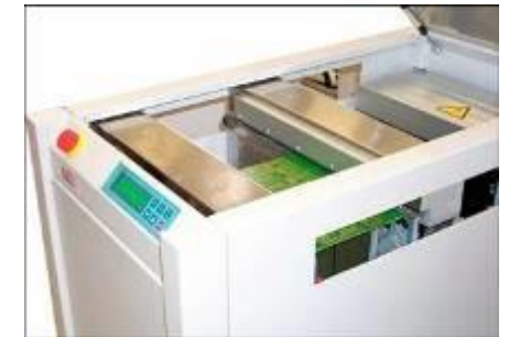
PCB is ready for handover to down-line machine
