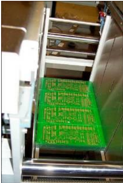
PCB stack placed on the stack table, ready to be processed
