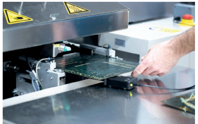
Reference board runs through the soldering system
