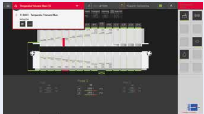
Alarm messages with a display of the action buttons and the favourites bar
