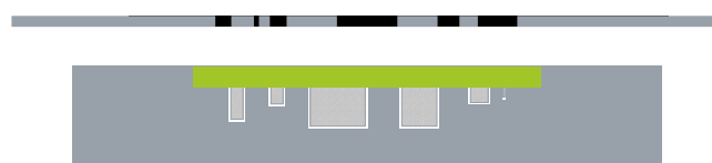
Single routed tooling plate to support side 1 and 2 (1st and 2nd pass tooling plate)
