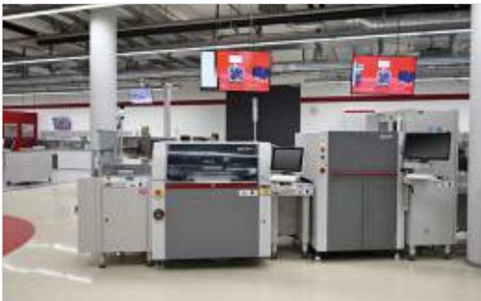
Real-life SMT lines in the SMT Centers of Competence are used to provide application support and run tests including SPI analysis.
