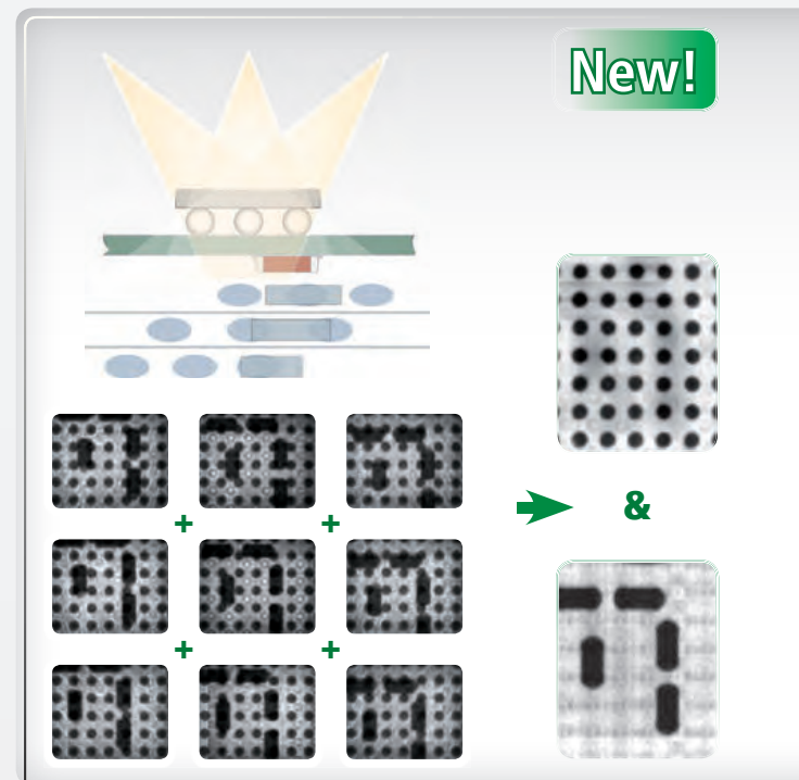
Different projections of a board with components on both sides during 3D X-ray inspection
