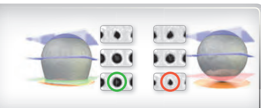
Detection of an un-soldered BGA ball in various layers of the solder joint
