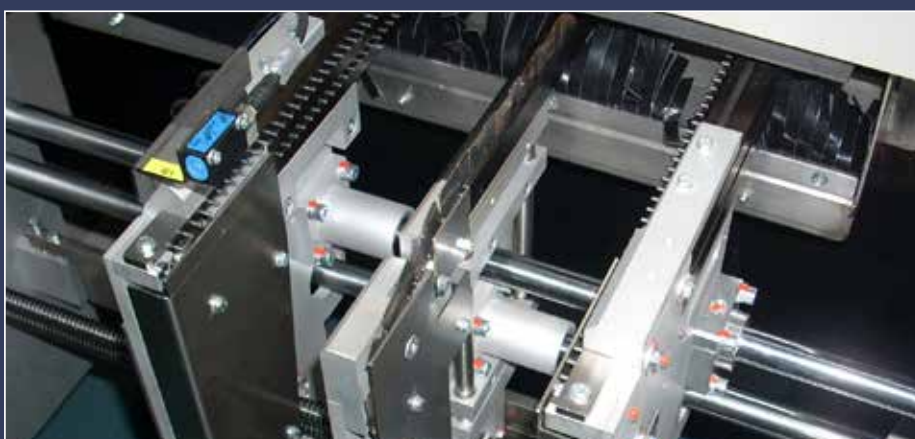
Single-lane conveyor with centre support
