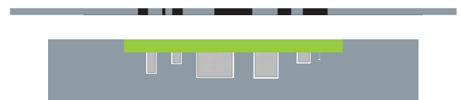
Single routed tooling plate to support side 1 and 2 (1st and 2nd pass tooling plate)
