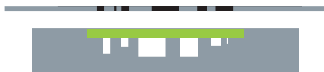
Single routed tooling plate to support side 1 and 2 (1st and 2nd pass tooling plate)
